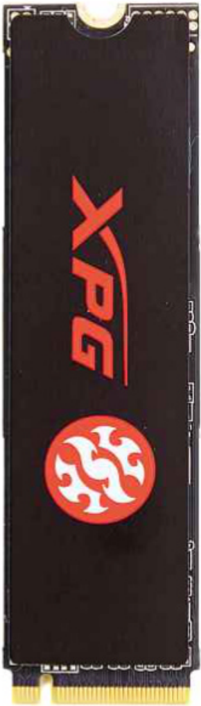
LEFT: An M.2 NVMe drive saves space and delivers the best performance
